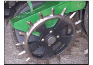
Spiked tooth press wheels for minimum till or no-till conditions.
